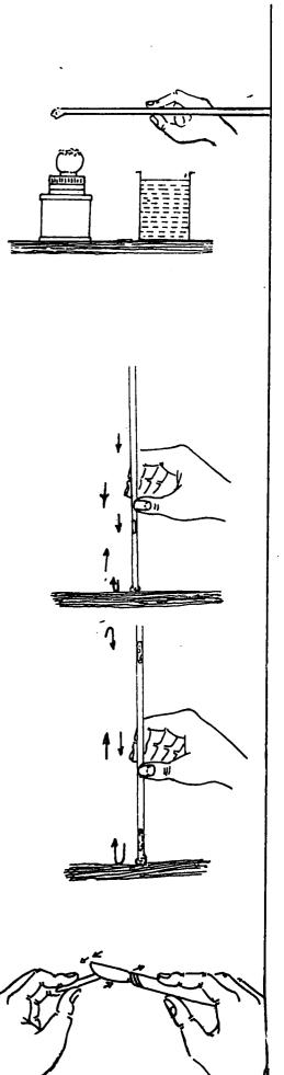
5. Drop 5 drops methylene blue indicator into each straw so that the filter paper is all wet. The blue colour should show clearly.
