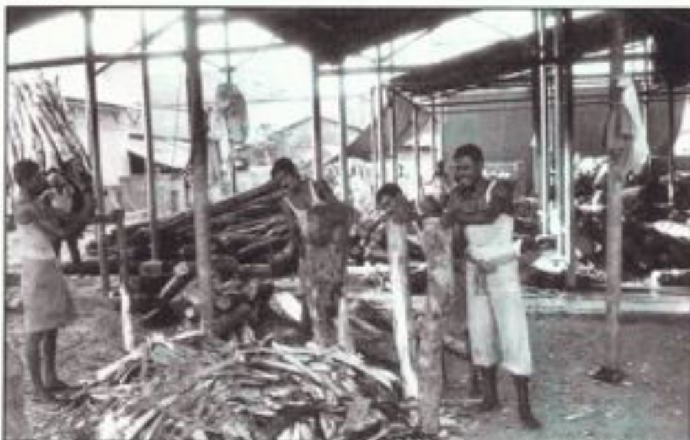
Khulna Newsprint Mill. Most barking is done by hand. Photo by Karlis Goppers/SIDA Photo Archives.
