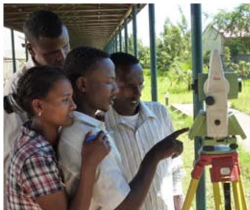
Surveyors learning how to use a “total station” surveying equipment
